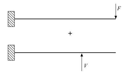
By clamping the beam, two of the three BCs of (b) are met, and V is the only unknown force. It is to be determined from the remaining BC that w(l) = 0:
